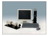
The semiconductor laser FFP measurement system uses a dedicated optical system and a digital CCD camera to acquire a 2D image of the beam spread angle of a semiconductor laser. The center of the acquired image represents the optical intensity at  $0^{\circ}$  versus the optics axis. The image at a position nearer the edge indicates the optical intensity at a wider beam spread angle.
